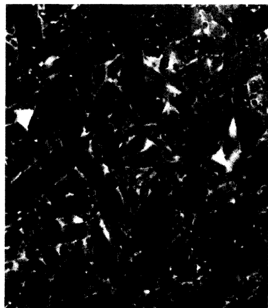
Fig. 2. Microstructure of the HP-Starck material hot-pressed.
